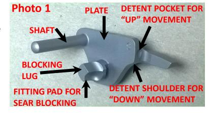
safety so that the blocking lug is hanging off of the rear of the frame tang, so only the shaft fit is being tested. The shaft should slide cleanly in to full depth. Should your frame have a too-tight pivot hole, open it slightly by using a chucking reamer that is the same decimal size as the shaft diameter. Turn it slowly with a variable speed hand held drill.
